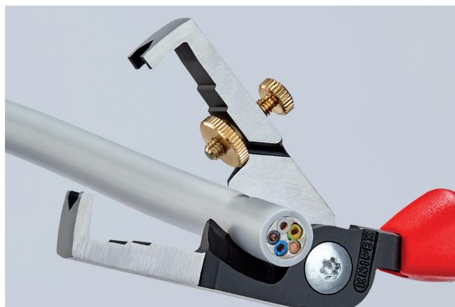
Induction hardened shear blade with precisely ground cutting edges for crushing-free cutting of copper cables up to Ø 15 mm (5 x 2.5 mm<sup>2</sup>)
